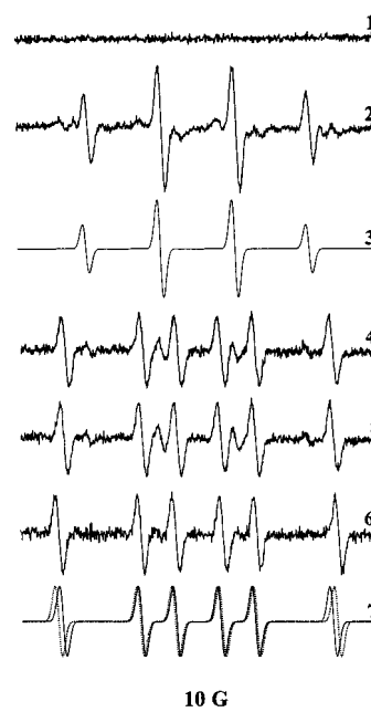
Figure 1. ESR spectra of DMPO nitroxides formed in a solution of AS. ESR measurements and spectra simulations were performed as described in ref 11. DMPO was used at a concentration of 0.1 M in phosphate buffer (pH 7.4, 25 °C). The hyperfine splitting constants (in G) used for simulation of the spectra of the DMPO/ \bullet\text{OH} , DMPO/HER, and DMPO/ \bullet\text{CH}_3 nitroxides were as follows: ( A_N = 15.0 ; A_H = 15.0 ), ( A_N = 15.8 ; A_H = 22.8 ) and ( A_N = 16.3 ; A_H = 23.2 ), respectively (11). AS was synthesized as described in (6). All ESR spectra were recorded after 2 min of incubation of the reaction solutions. Spectra 1 , no addition; spectra 2 , plus AS (0.1 mM; a stock solution of AS was prepared in 0.2 M NaOH); spectra 3 , computer simulation of the ESR spectra of DMPO/ \bullet\text{OH} ; spectra 4 , plus ethanol (0.5 M) and AS; spectra 5 , ethanol and AS were added after deoxygenation of all solutions with \text{N}_2 for 45 min; spectra 6 , plus DMSO (0.3 M) and AS; trace 7 represents computer simulation of the ESR spectra of DMPO/HER (solid lines) and DMPO/ \bullet\text{CH}_3 (dashed lines). The ESR spectra in repetitive experiments did not differ more than 10% ( n \geq 3 ).
